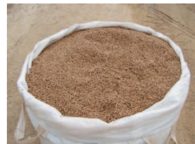
Finished switchgrass pellets – Stored in 1-ton mini-bulk bags
